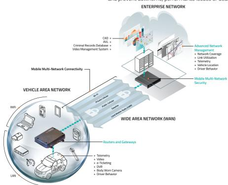
Connection Manager (ACM), the MG90 consolidates the security for all connected technologies in the vehicle area network (VAN), vastly simplifying deployment and enabling the enterprise to retain management control over network access and connected mobile assets.
